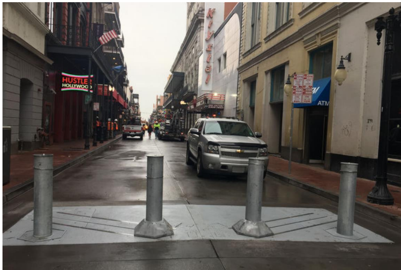
Matador Surface Mount Automated Bollard System Pedestrian & vehicle permeability – 2 middle bollards move on sliding tracks (manual). Permanent installation.
