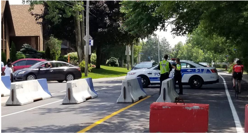
Pedestrian permeable HVM design solution integrated with vehicle & traffic control checkpoint at a local festival Montreal, QC
